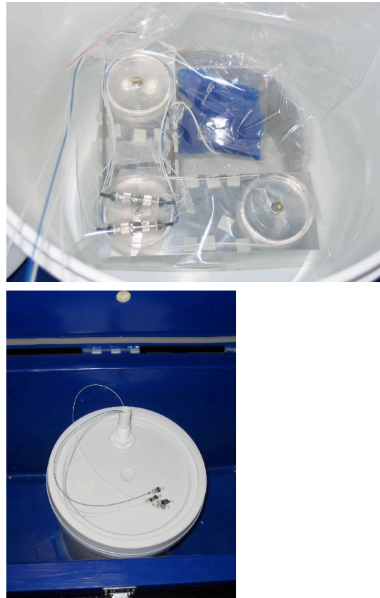
Fig. 4: (a) Detectors are horizontally located inside an air-filled bucket. The plastic bag reduces even further any air movements, and thus temperature differentials. The blue crystals are silica gel to reduce moisture. (b) Bucket located inside and attached to bottom of the insulated container prior to adding water to the container.
