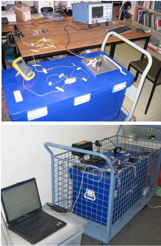
Fig. 3: (a) Detector 1 (D1) is located inside a sealed air-filled bucket inside an insulated container (blue) containing some 90 kg of water for temperature stabilisation. This detector, in the School of Chemistry, Physics and Earth Sciences, had an orientation of 5^\circ anti-clockwise to the local meridian. Cylindrical He-Ne laser (Melles-Griot 0.5 mW 633 nm 05-LLR-811-230) is located on LHS of bench, while data logger is on RHS. Photodiode detector/pre-amplifier is located atop aluminium plate. (b) Detector 2 (D2) was located 1.1 km North of D1 in the Australian Science and Mathematics School. This detector had an orientation of 11^\circ anti-clockwise to the local meridian. The data was logged on a PC running a PoScope USB DSO (PoLabs http://www.poscope.com ).
